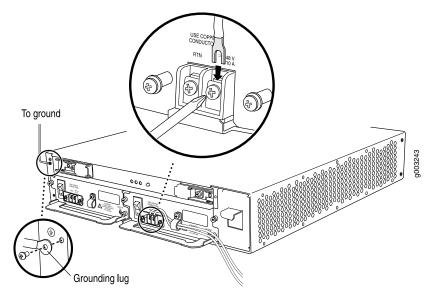
Figure 6: Connect the Power Cables to a DC Router
